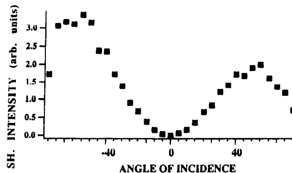
Figure 5. Plot of angle of incidence vs SH intensity of spin-coated film of poly(BPOD).
